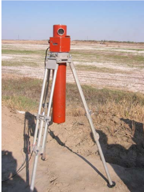
Photo 7. A rotating laser light source.
