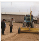
Laser-assisted land leveling, an innovative technique saving water up to 25-35%, forms a part of Uzbekistan's national agriculture development plan for 2014-2020, deriving from SLM research of ICARDA and its partners, and funded in part by ADB.
